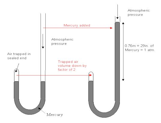
Boyle found that when more mercury was poured into the tube, increasing pressure on the trapped air, the air volume halved if the *total* pressure, including that from the atmosphere, was doubled.
